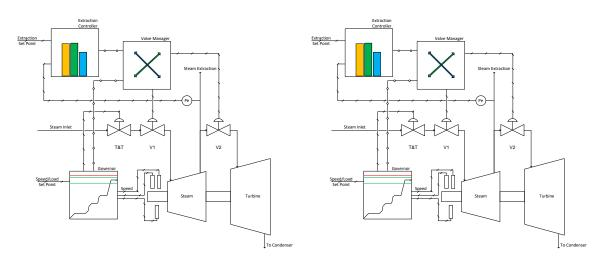
The Tri-STIG has extremely high availability, 2003 Triple Modular Redundant architecture, allowing module replacement and design modifications even with the Turbine running.
